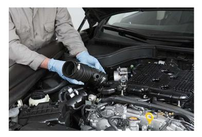
4. Remove the air intake duct.
