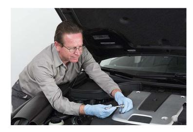
1. Remove the engine cover nuts and bolts.
