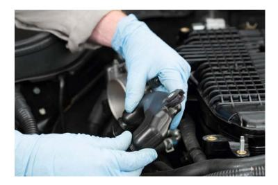
7. Move the crankcase ventilation chamber off to the side.
