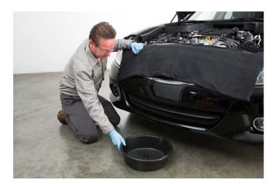
5. Place a drain pan under the vehicle to catch any coolant.
