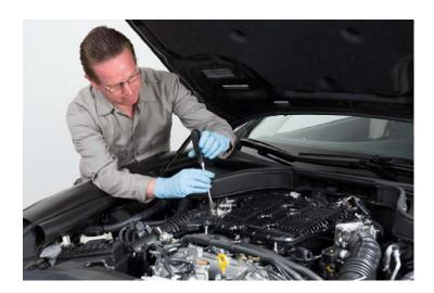
3. Loosen the air intake duct clamps.
