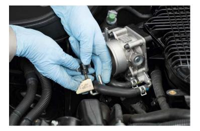
8. Clamp off the coolant hoses to the throttle body.
