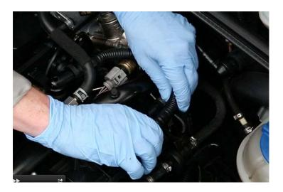
9. Remove the PCV hose by squeezing the clips while carefully wiggling the hose out of the fittings.
