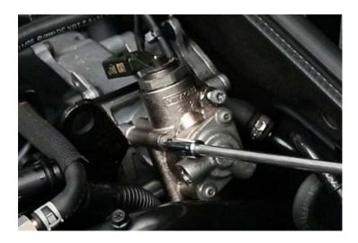
14. Remove the 3 bolts for the high pressure fuel pump.
