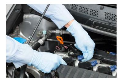
2. Disconnect the ignition coil connector.
